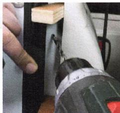
12 -Percer Ø 5 Monter Bague Ralonge & Poser le 1er Rivet
